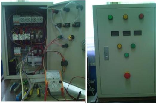
Gambar 9 Modul Sistem Kontrol ATS Hybrid
